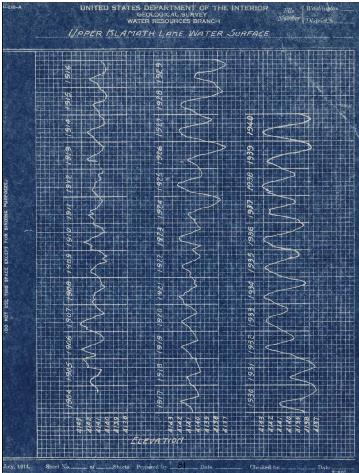
Figure 5. U.S.G.S. Recorded Upper Klamath Lake Elevations 1904-1940. Note UKL Elevations in alongside historical evidence of the Link River being Dry in 1908, 1911, and 1918.
